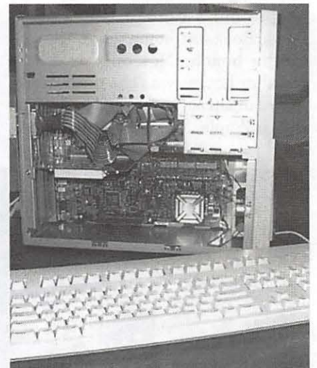
On the inside, the Motorola StarMax begins to look more like a Macintosh, starting with the green fiberglass motherboard adorned with "© Apple Computer Inc." printed right on it. By the end of the year, Motorola should be selling StarMax machines without the Apple copyright, based instead on Motorola's version of the CHRP (Common Hardware Reference Platform) design. But you'll still be able to run MacOS.
