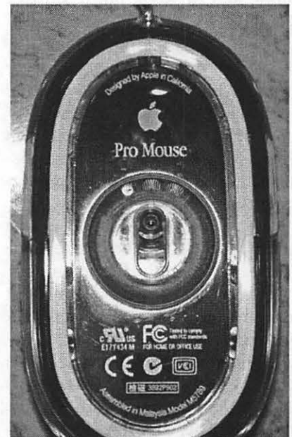
Look, Ma, no rollers or ball! The bottom of the mouse does reveal a "Designed by Apple in California" label, and also mentions it was "Assembled in Malaysia." Note the three-position adjustment ring around the optical sensor in the center. (Photo by Lawrence I. Charters)
