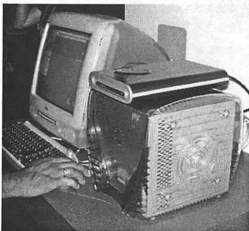
The MicroNet SANcube offers up to 270 billion bytes of storage in an attractive box that can be hooked up, via FireWire, to four Macs. The unit sitting on top is a separate tape backup unit. (Photo by Lawrence I. Charters)
