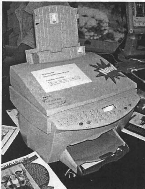
It may look funny, but the Hewlett-Packard OfficeJet G85 combines an inkjet printer, scanner and fax machine in one unit. (Photo by Lawrence I. Charters)
