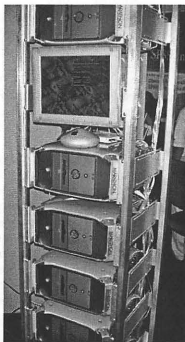
Marathon sells metal brackets that replace the plastic handles on G3 and G4 towers, allowing them to be mounted in standard LAN racks. This particular stack of five G4 Macs, complete with a liquid crystal display, attracted lots of attention from networking personnel. (Photo by Lawrence I. Charters)
