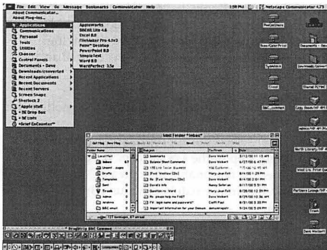
Figure 5 – A screen capture of my Desktop. Note the accessibility of applications under the Apple menu in the upper left and the DragStrip along bottom left. The right side shows the mounted, shared folders (the ones with the “tail”), Desktop Printers, folders and hard disk.
