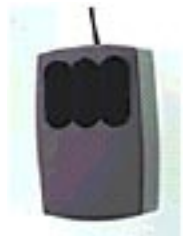
THREE TO ONE: Apple decided that the mouse for the Lisa should have fewer buttons than the Xerox PARC mouse. Courtesy Dean Hovey
