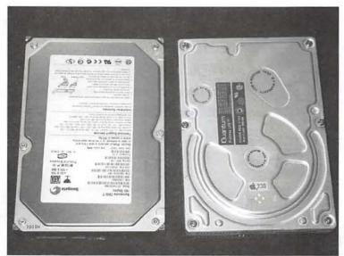
Step Two: marvel at changes in technology. The drive on the left is a brand-new Seagate Technologies 160 billion byte Barracuda serial ATA hard drive, purchased for \$100 in February 2004. The drive on the right is a Quantum ProDrive LPS 230 million byte SCSI drive originally bundled with (we think) a Power Mac 7200. (Photo by Lawrence I. Charters, taken with a Canon PowerShot G3 digital camera.)
