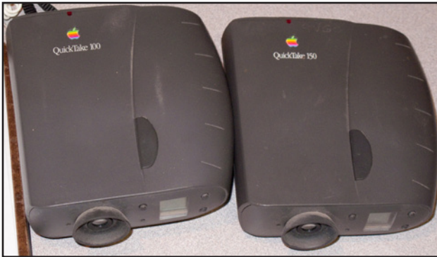
Two of the three Apple QuickTake cameras. These were not the first digital cameras, but their introduction greatly boosted the adoption of “consumer” digital cameras. The QuickTake 100, on the left, was introduced in 1994; the QuickTake 150 in 1995. Both were designed by Kodak, built by Chinon Industries. Photo by Lawrence I. Charters.
