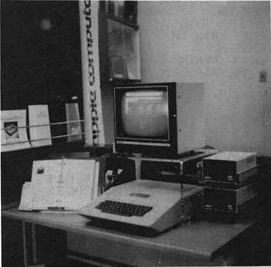
**VERSA-STAND.** Constructed of  $\frac{3}{8}$ " clear acrylic with cutouts providing good ventilation for the terminal. Two disk drives can be placed on top of the terminal. For easy access to the peripheral cards place the drives on side shelves. The desk space is still free for other equipment. A third shelf can be mounted on the left side to hold other accessories such as a disk file. Brackets can also be provided for various attachments.
