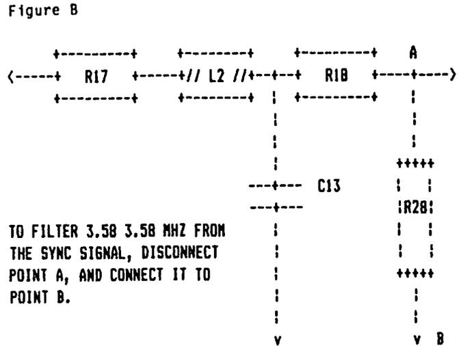
Schematic Diagram of the Apple II PAL Color Encoder Card
