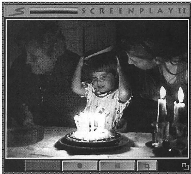
**The Big Window:** ScreenPlay II comes with Spigot II Tape and serves as a video capture and playback application. This window, at 320x240 pixels, is the biggest size you can get full-motion video with Spigot II Tape. With the right computer you can make 30 frames per second movies, though most Macs capture at slower rates. (This is my daughter Claudia's second birthday party.)
