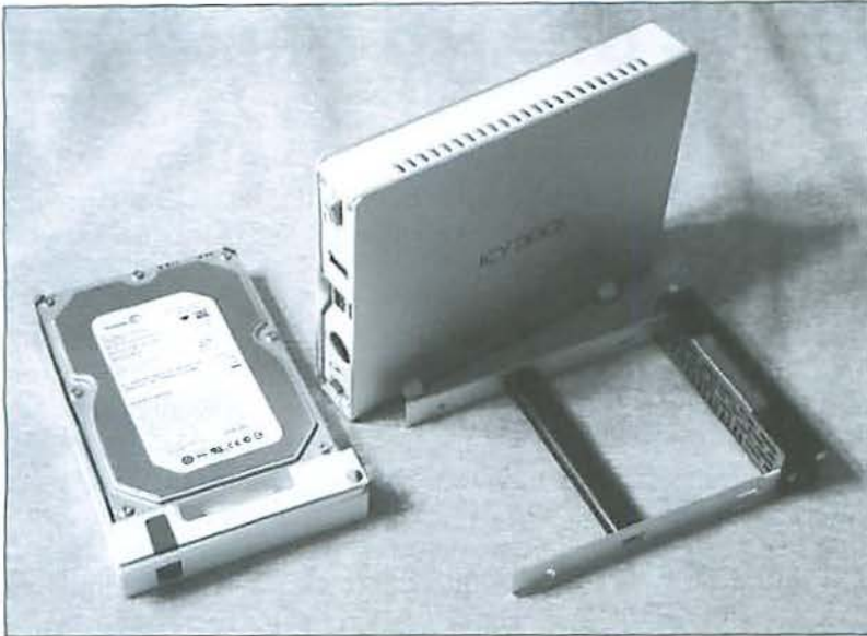
An ICY DOCK drive enclosure, drive bracket, and Seagate drive mounted in an ICY DOCK bracket. ICY DOCK enclosures come in various flavors including USB 2.0, FireWire 400, FireWire 800, and combinations of USB 2.0 and FireWire. Photo by Lawrence I. Charters.
