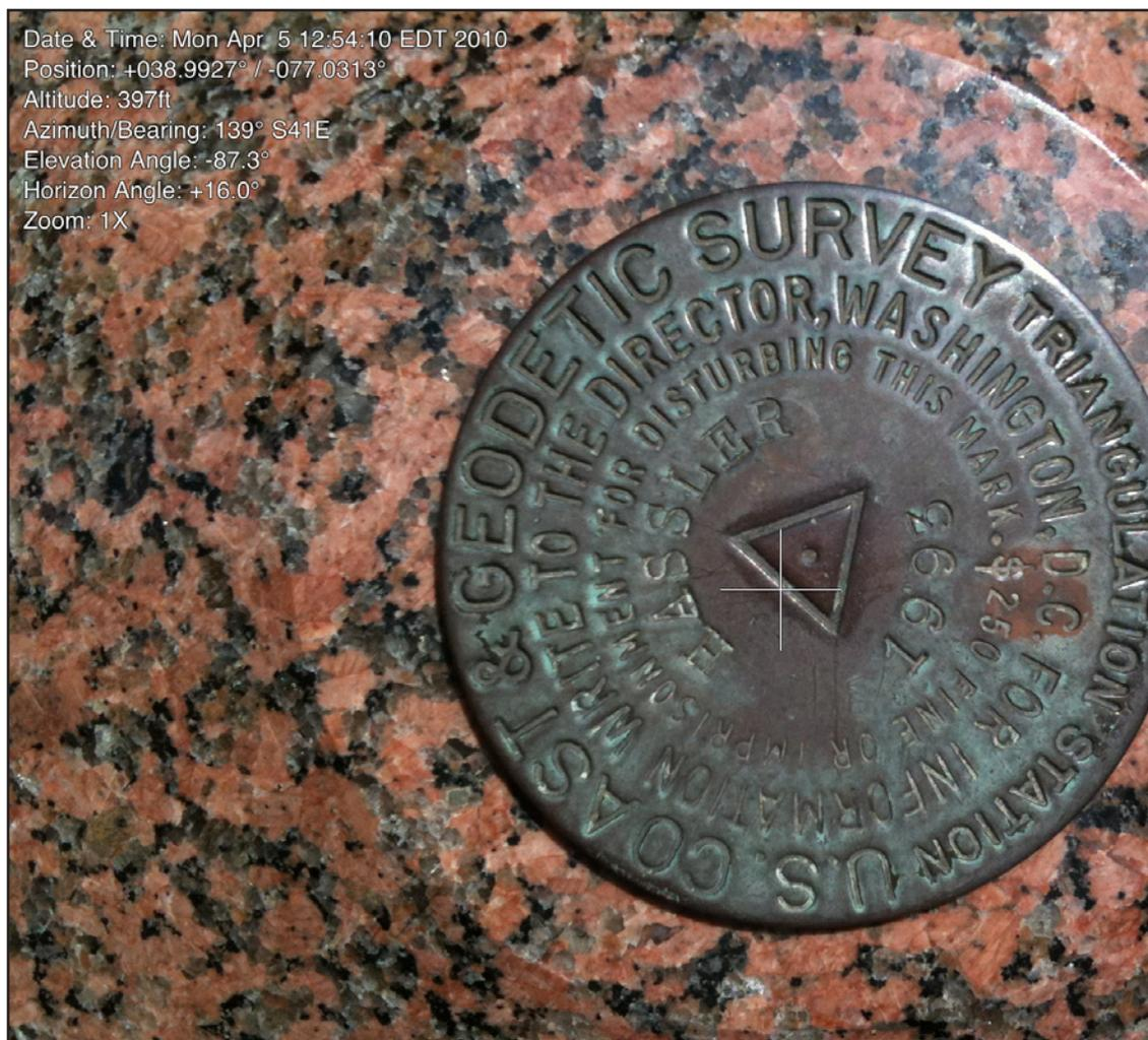
**Figure 3:** The Hassler Triangulation Station survey marker, shot from directly overhead with *Theodolite*. Overwritten on the image is the time and date, a position of +038.9927°, -077.0313°, an altitude of 397 feet, azimuth/bearing of 139° S41E, elevation angle of -87.3°, horizontal angle of +160°, and no zoom. The information is displayed slightly differently here than in the photo of the Pi offices, taken four months earlier, thanks to updates from the publisher.
