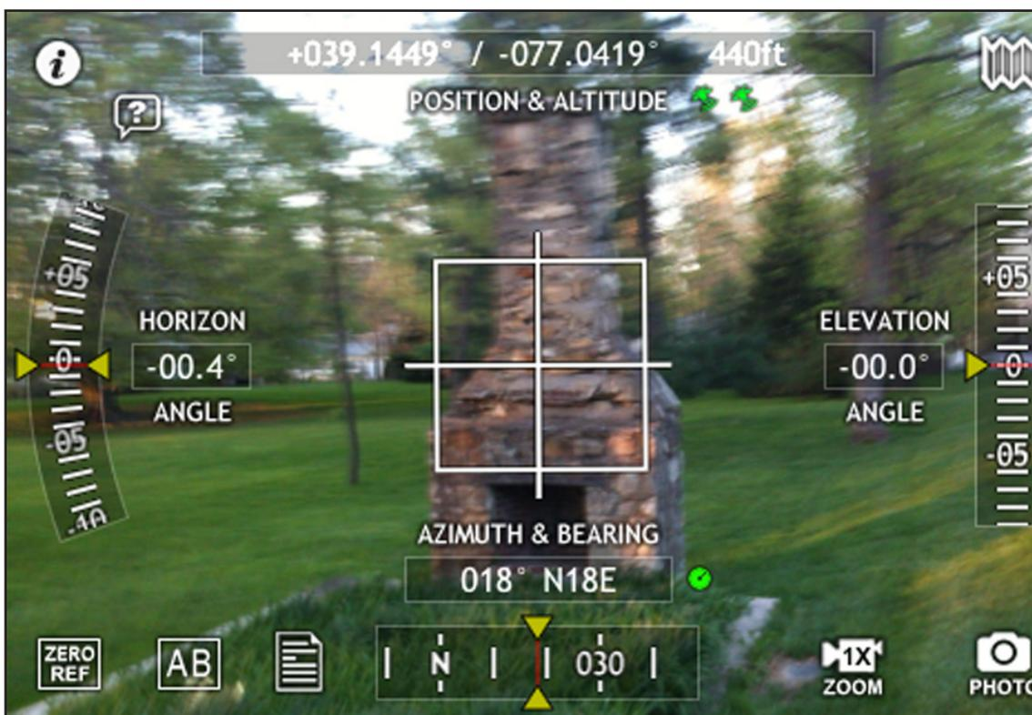
to: bring up a screen for adjusting settings and doing calibrations; launch Safari so you can read the documentation on Hunter's Web site; launch *Google Maps*; zero reference your settings; determine distance via A/B references; “zoom” the camera; and (the button in the lower right corner) take a photo.
