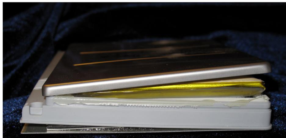
Seen from one end, the bottom plate is separated from the case and pushing down, while the inner shell has separated and is pushing up. This represents a considerable amount of force but, remarkably, neither the user nor the MacBook Pro was harmed.
