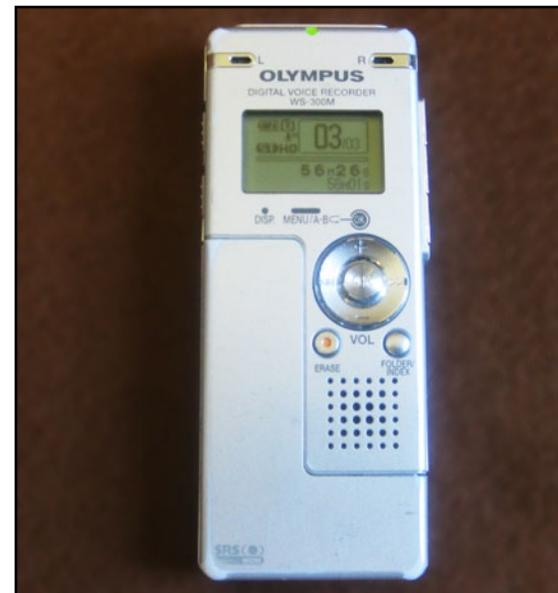
**Left:** The small Olympus WS-300M recorder works great for recording meetings. When it comes time to download the file, the battery pack detaches to reveal a USB connector which attaches directly to the computer. No wires, no fuss.
