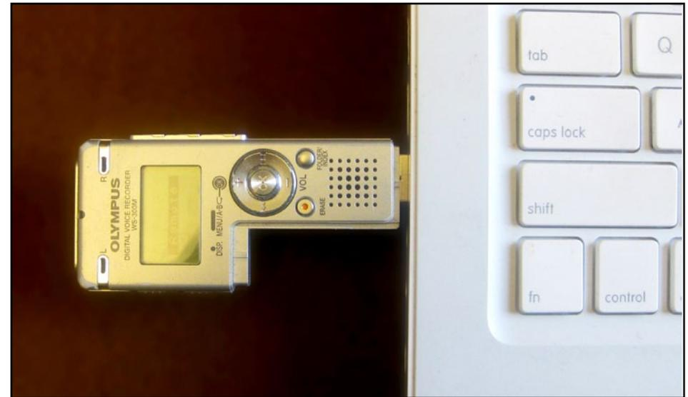
**Above:** The Olympus WS-300M digital recorder mated to a MacBook for uploading the recorded sound file. The recorder easily disassembles and then cleverly attaches via the Mac's USB port.
